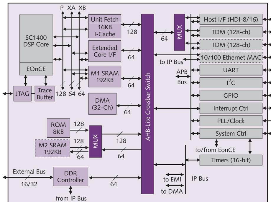
**Figure 2.** Rich in on-chip memory and peripherals, the Freescale MSC711x-series chips are the first DSPs with glueless DDR SDRAM controllers. Other members of the family are minor variations of this MSC7116 design, generally having less on-chip memory, fewer time-division multiplexers, and, in some cases, omitting the Ethernet controller.
