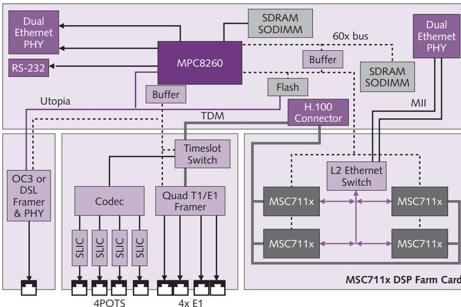
**Figure 1.** This VoIP reference design (available from Freescale later this year) uses four MSC711x-series StarCore chips on a "DSP farm card" to assist a PowerQuicc II MPC8260 communications processor. Such a system might be capable of handling 64 premium-voice channels or more than 100 G.711 channels.
