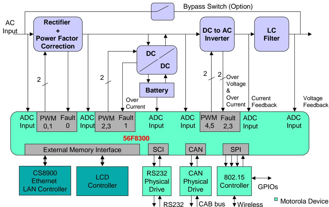
**Figure 2-1. Network-enabled UPS Hardware Diagram**
