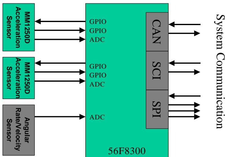
**Figure 2-9. Intelligent Inertial Sensor with Three Variables**
